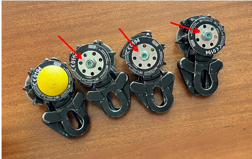
Photo 5: Multiple missing yellow buffers on multiple Transfasteners. TYP.
