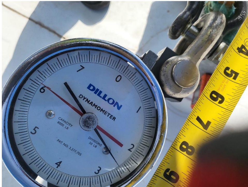
Photo 2 – A calibrated dynamometer gauge with a test load of 2,500 lbs.
